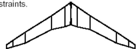
E Minimum total drag, fixed weight, low speed lift constraints, fuel inertia relief, and static aeroelasticity.
