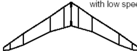
D Minimum total drag, fixed weight, low speed lift constraints, and fuel inertia relief.
