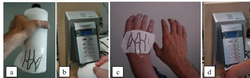
Figure 5-27: Vascular pattern spoofs effective with liveness detection turned off. a) The copy of a vascular pattern stuck on a bottle. b) The bottle spoof verified as an authorised user. c) The copy of a vascular pattern stuck on a hand (left), next to the original hand (right) of an authorised user. d) The hand spoof verified as the authorised user
